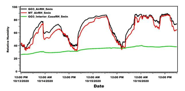
Figure 4. Time series of relative humidity from the GO3 and Moody Tower systems. The interior RH for the case is for housekeeping purposes and the progressive increase over time is addressed in more detail below.
