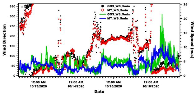
Figure 5. Time series of wind speed and wind direction from the GO3 and Moody Tower systems. It should be noted that the Moody Tower uses a propeller and vane anemometer and the GO3 uses a compact integrated met sensor with 2-D sonic anemometer.
