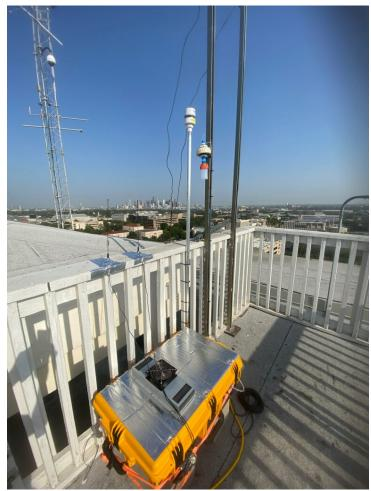
Figure 1. GO3 sample box on the roof of a Moody Tower lab trailer with met sensor and inlet. The main Moody Tower (C695) sample mast is in the background where  $O_3$  and met parameters are measured for C695.
